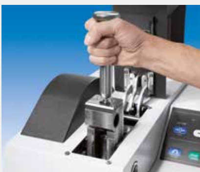
Easy removal of the crushing arm without tools
