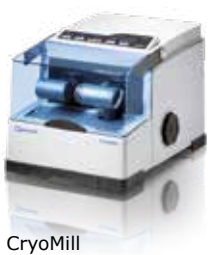
Material embrittled with liquid nitrogen
