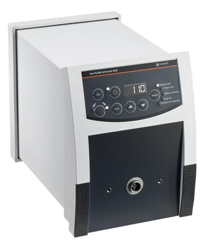
The ability to switch between precise dosing and fast conveying make this pump model the perfect complement to a reactor system. With a flow rate of 2.0 - 4,056 ml / min, when operated with single-channel pump heads, flows from feed-batch and chemostat modes of operation can be conveyed precisely. Rapid filling and emptying of the reactor system is also possible.
