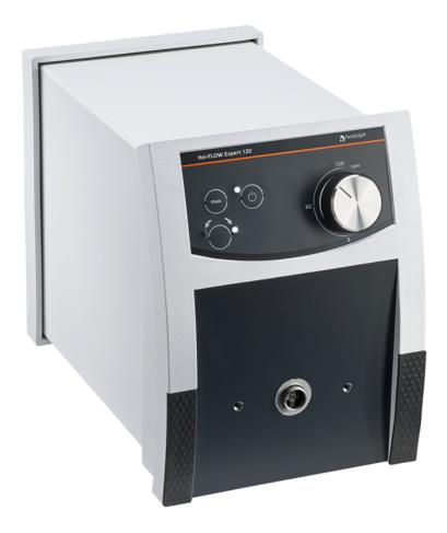
The pump drive of the model 120 of the Hei-FLOW Expert series can be operated with either single-channel or multi-channel pump heads. The flow rates with single-channel pump heads are in the range of 0.38 - 813 ml/min; with multi-channel pump heads from 0.005 - 329 ml/min.
