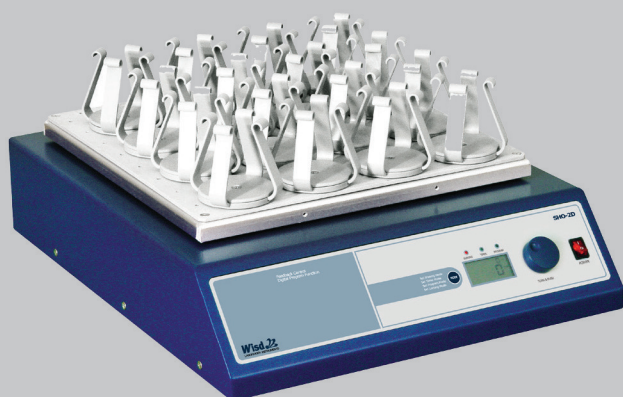
SHR-2D with optional universal platform and flask holder
