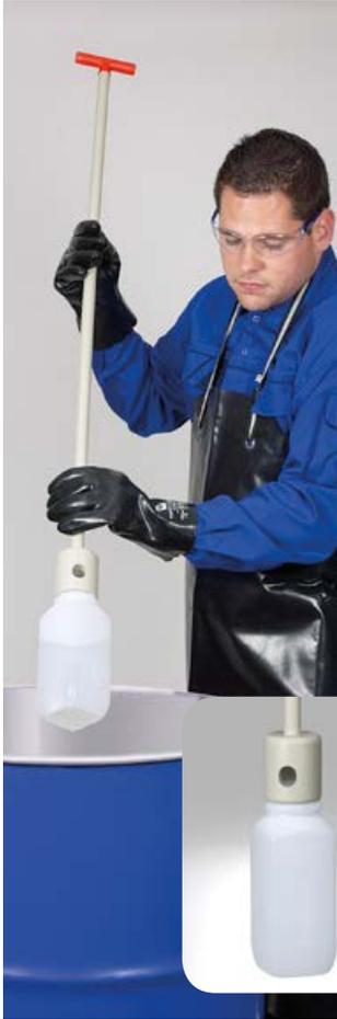
The ChemoSampler was developed for sampling aggressive liquids, e.g. acids, alkalis, detergents. The samples are drawn directly into the screw-on original sampling bottle. The tamper-proof bottle closure of these bottles with original safety ring ensures unadulterated sample transport. Samples can be taken from depths of as much as 200 cm, e.g. from tanks, silos or tankers, by using the extension rod.
