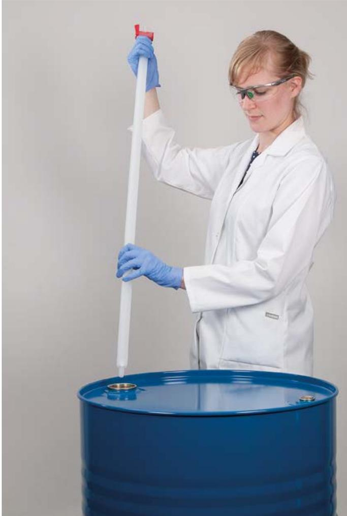
Dip sampler for simple removal of liquid samples. Good view due to transparent tubes. Upper end with reflux valve, lower end with ball valve.
