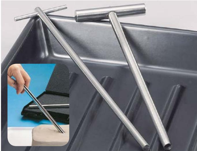
Cylindrical hollow drill with a sharp cutting edge, can easily be driven into paste-like and semi-solid substances. The samples cut out are subsequently removed with the appropriate push-rod ejector. Total length 260 mm. Inner Ø 8 mm, outer Ø 10 mm.
